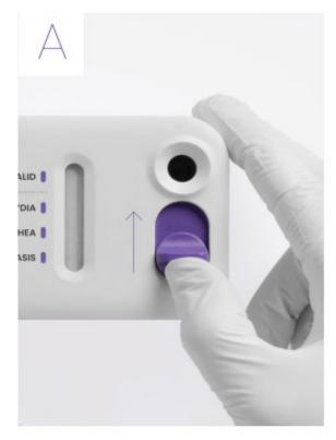
Immediately after sample addition, slide the **switch upwards** in a firm, swift motion to fully close the sample port and ensure the test is started.
