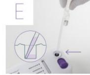
Place the tip at the **bottom** of the sample port and then squeeze the **upper bulb** of the pipette to release **all** of the sample.
