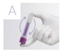
Mix the sample (or control) by **gently inverting** the tube **5 times**.
